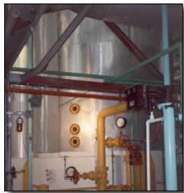
**Evaporation** – The clarified juice is then boiled in evaporators which remove most of the water leaving a thick syrup.
