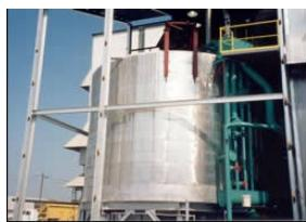
**Clarification** – The raw juice is strained and heated. Lime is added to cause impurities such as mud to settle. Clarifiers separate the juice into clarified juice and muddy juice. The muddy juice is sent to filters where any juice is removed leaving mud (filter cake) which is returned to the fields.
